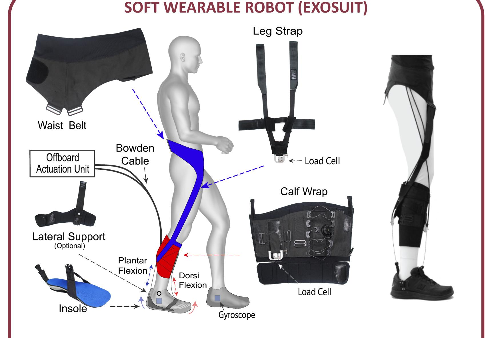
Reductions in paretic hip <u>circumduction</u>  $(-20 \pm 5\%)$  and <u>hip hiking</u>  $(-27 \pm 6\%)$ observed when comparing exosuit unpowered to powered conditions.
