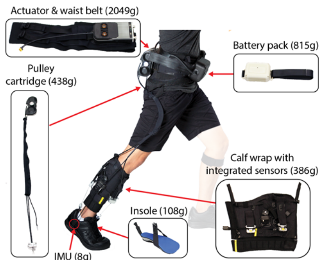
Figure 2. Exosuit hardware components and their masses
